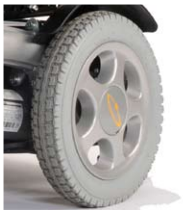
Solid / Pneumatic Knobbly Drive wheels
